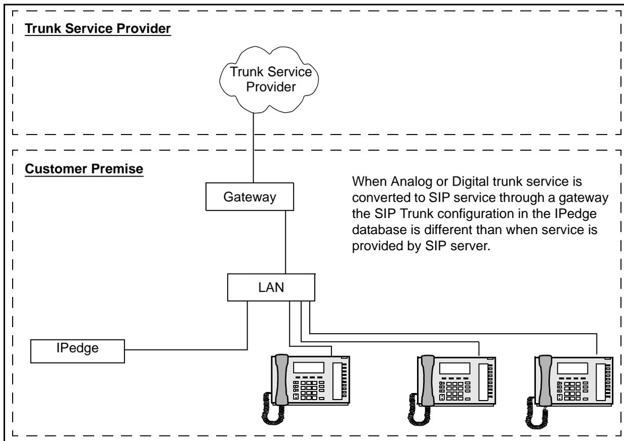
Figure 2 IPedge System with SIP Gateway
