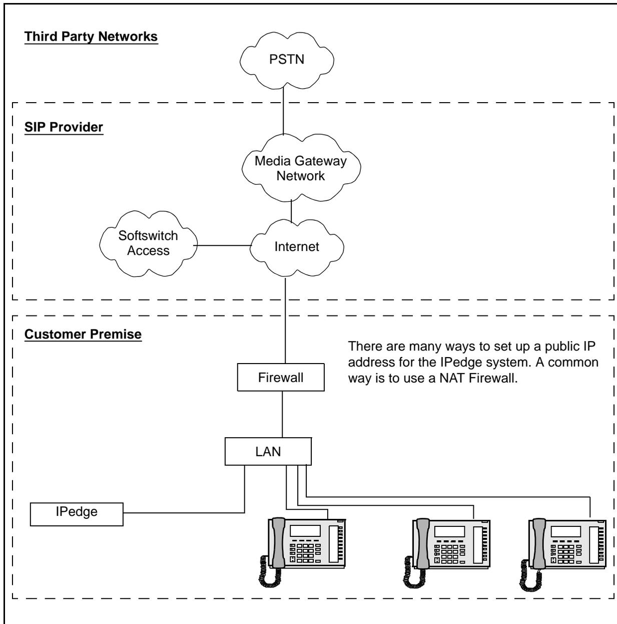
**Figure 1 IPedge System with SIP Trunking**
